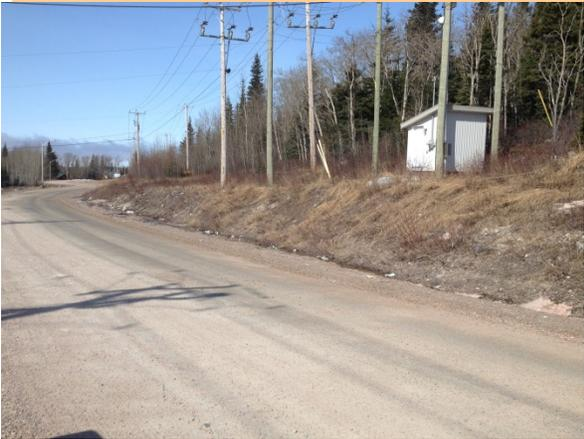
Photo 60: 1+200 Culvert required if rock is excavated from the ditch
